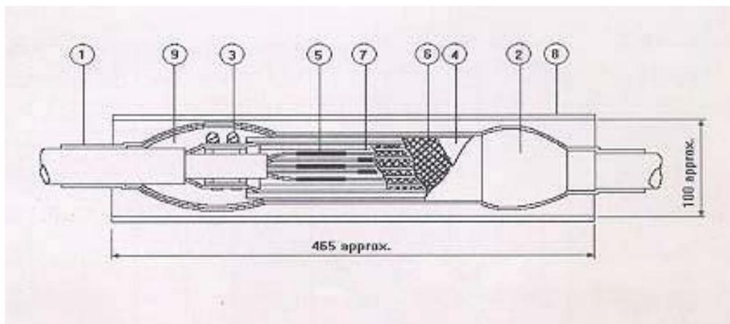
1. **P.I.B. Self-Amalgamating Tape** - provides electrical strength
