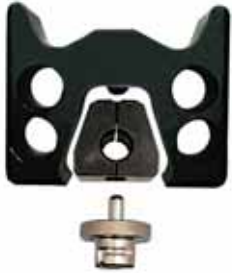
Matrix holder V2521, matrix P13M, punch P13D.
