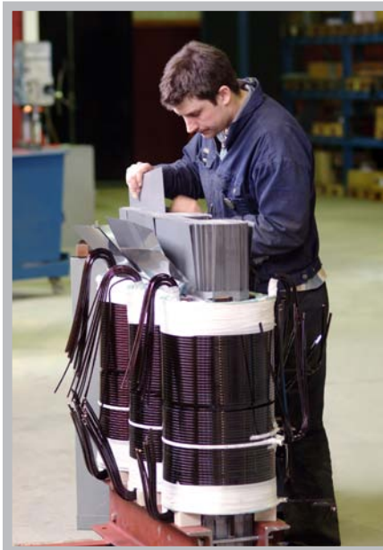
Low voltage transformers
